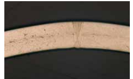
Narrow Viega laser weld seam
